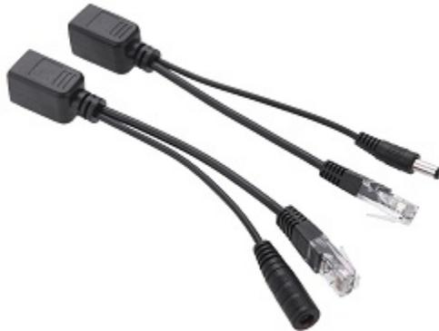
The next development phase still would use a similar adapter above, but only on the camera side. They would then connect the other end of the cable into a network switch that had 48V being sent to the camera, but the adapter would knock it down to 12V as to not harm the camera. This is what one PoE switch looks like.
